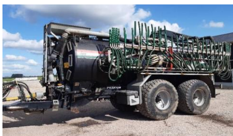
PEECON BJ 2013 EUR- 200, Kranarm, 24m Schleppschlauch, 750/60 R30,5
